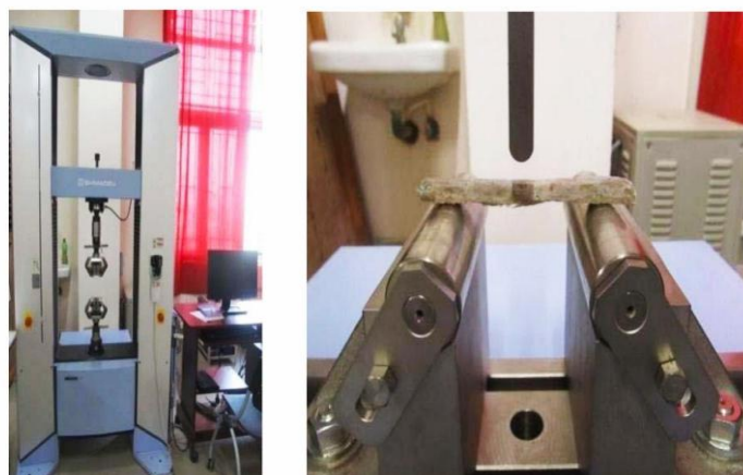
Figure 3. (a) Universal testing machine; (b) Flexural test setup
